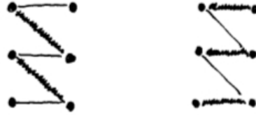
Fig. 1. The matching (thick edges) on the left-hand side is maximal but not maximum. The right-hand side shows a maximum (and perfect) matching in the same graph.
